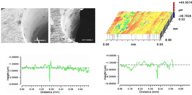
Fig. 2 Top row: surface quality of the holes drilled with SD and WD (left – SEM images showing drilled holes, right – surface roughness plot obtained using Zygo interferometry). Bottom row: Left – surface roughness profile of the hole using SD, right – surface roughness profile of the hole using WD.
