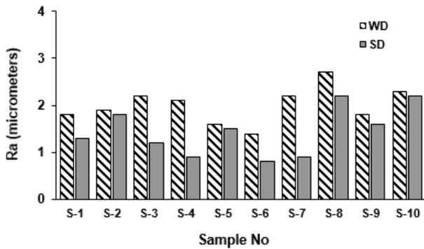
Fig. 3 Surface roughness of the drilled holes in 10 samples.
