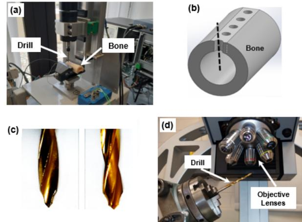
Fig. 1 (a) bone drilling system with necessary attachment for force and temperature measurements, (b) bone specimen for drilling, (c) surgical drills, (d) surface roughness measurement system for drills.
