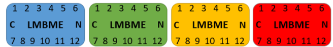
Fig. 2 Colour-coded PM stickers. Each colour represents a calendar year, repeated every four years. The numbers represent the month that PM was last completed and should be punctured accordingly. The “C” and “N” markings pertain to PCUs. The “C” is punctured when its battery is conditioned, and the “N” indicates that a new battery was installed that year.
