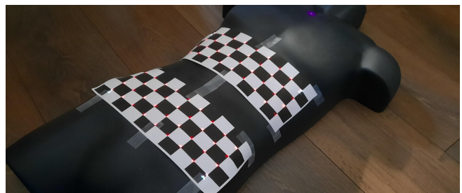
Figure 3: Image of checkerboard saddle points projected onto the surgical mannequin. This provides a visual representation of the reprojection error.
