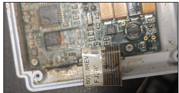
Figure 4 Failed Internal Battery due to liquid infiltration
