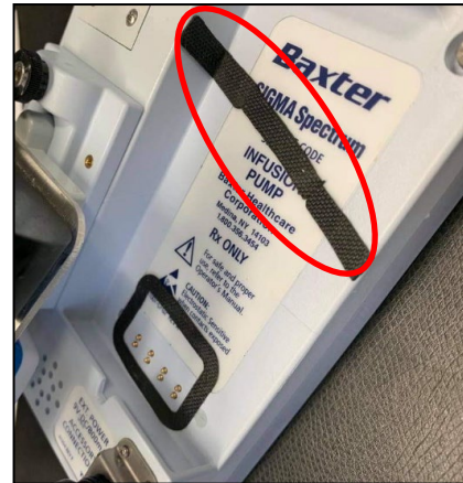
Fig. 8 Installation of a second gasket barrier
