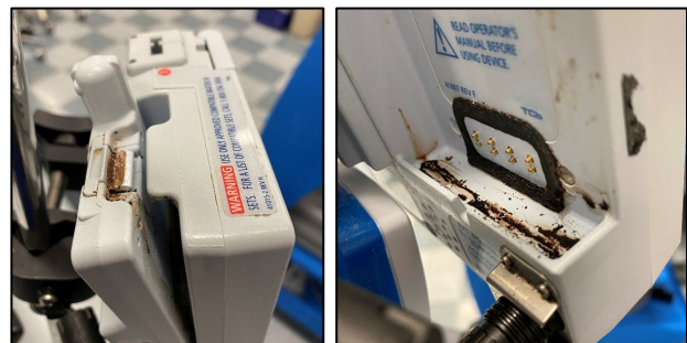
Fig. 5 Fluid Invasion between Pump Case and Battery Module
