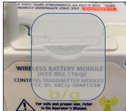
Fig. 10 Installation of a tape over the battery lock
