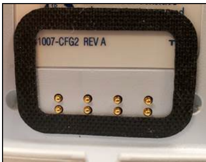
Fig. 7 Installation of a new foam gasket
