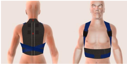
Fig. 1 The designed orthosis, (red: inertial sensors, dark gray: Electrodes)
