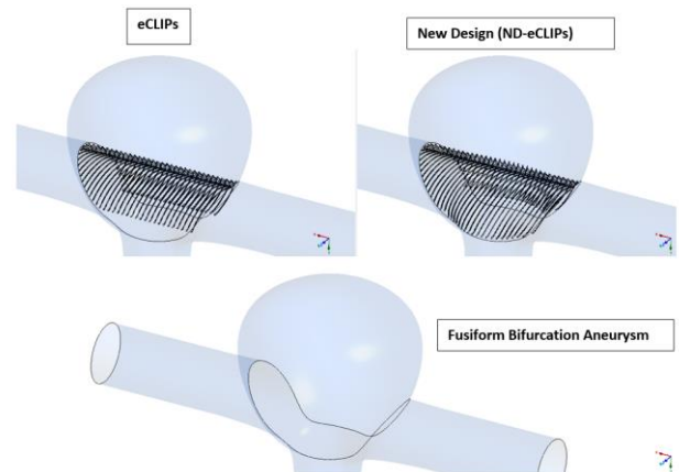
Fig. 1 Geometry of the fusiform bifurcation aneurysm with the eCLIPs and New Design implanted at the neck
