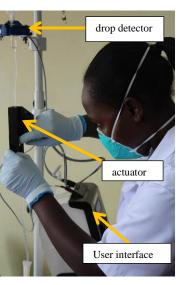
Fig. 1 Features of the ECGF device
