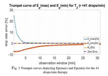
Three runs were recorded during the 41 drops/min therapy that ran for a total of 227 minutes as shown in Table 1. Since there were no continuous runs for more than two hours without alarm interruptions, trumpet curves for  $T_1$  are similar to those of  $T_2$ . The maximum error for this infusion therapy was an E\_total of 4.065%.
