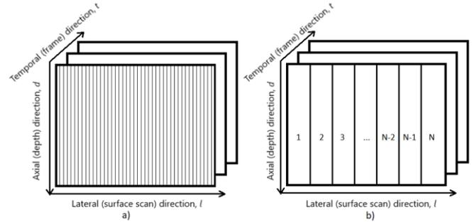
Fig. 2 Structure of the acquired ultrasound RF signal data a) with 127 lateral RF signals and b)  $N$  averaged RF signals.
