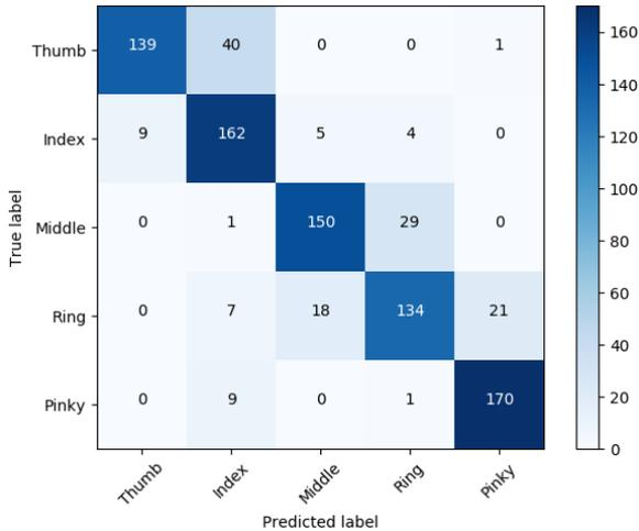
Fig. 6 Confusion matrix for  $N = 4$  reconstructed RF signals.
