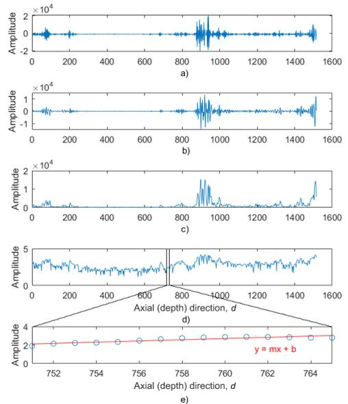
Fig. 3 Preprocessing and feature extraction on a) raw RF signal acquired, b) normalized and Gaussian filtered signal, c) envelope of signal, d) log compression, and e) linear fit features extracted using linear regression.
