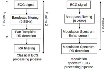
Figure 2: RR series extraction pipelines explored herein
