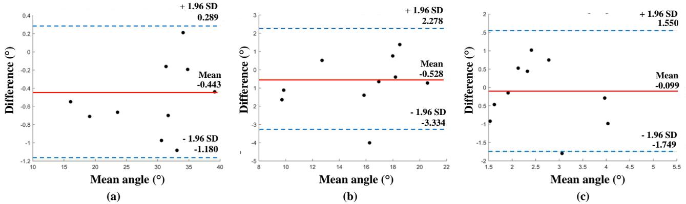
Fig. 1 Bland-Altman analysis for relative range of motion measurements between IMUs and Vicon. (a) Flexion-extension. (b) Lateral bend. (c) Axial twist.
