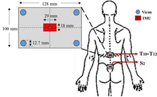
Fig. 1 Sensor configuration and placement.
