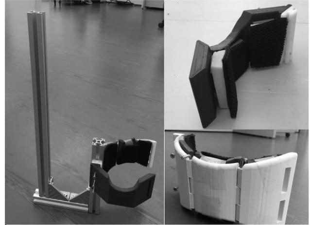
Figure 1. Prototype transtibial adaptor. Left shows the custom designed cuff mounted on the aluminum frame. Top-right shows front plate. Bottom-right shows adjustable back plate.
