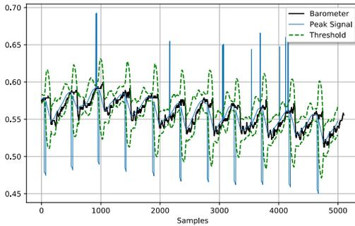
Fig. 3: Z-score algorithm applied: peak detection from the raw data
