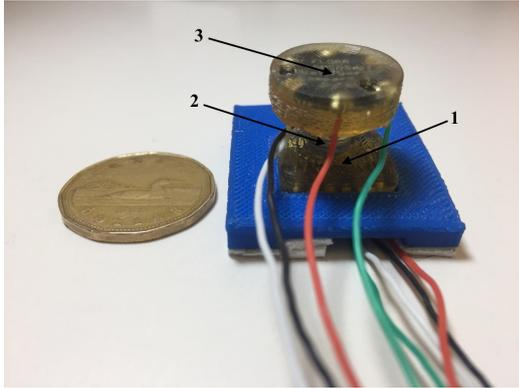
Fig. 1: The Multimodal Tactile Sensor: 1 - MARG (Magnetic, Angular Rate, and Gravity) system; 2- Cone compliant structure 3 - Shallow barometer
