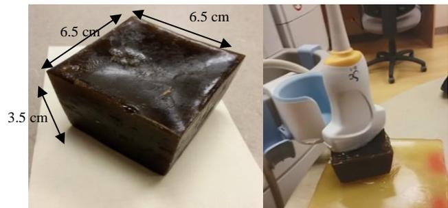
Fig. 1 Left: Phantom with its dimensions. Right: Ultrasound Transducer on the phantom for image acquisition.
