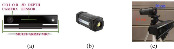
Fig. 2. Imaging devices and their assembly: a) Kinect Xbox One color and depth sensors, b) FLIR A320 infrared camera, and c) assembly of multispectral sensor for a subject located on the right side.
