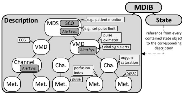
Fig. 2. Schematic overview of device capability modeling (example containment tree; speech bubbles contain example content)
