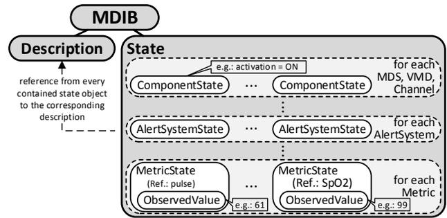
Fig. 3. Schematic illustration of selected (partial) states of the device state (speech bubble contain example values)
