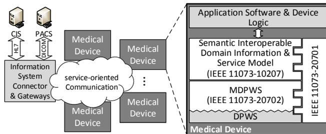
Fig. 1. Schematic overview of the device communication and the new IEEE 11073 Standards
