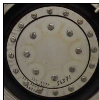
Figure 2: Heat stress star pattern on driver faceplate
