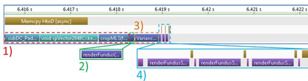
Figure 1. CUDA processing pipeline captured using the NVIDIA Visual Profiler.
