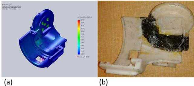
Figure 4 – (a) Elbow joint structural analysis (b) Reinforcing with carbon fibre wrapping
