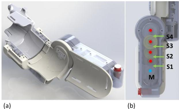
Figure 1 - (a) RAO (b) M-motor, S#-stage 1 to 4
