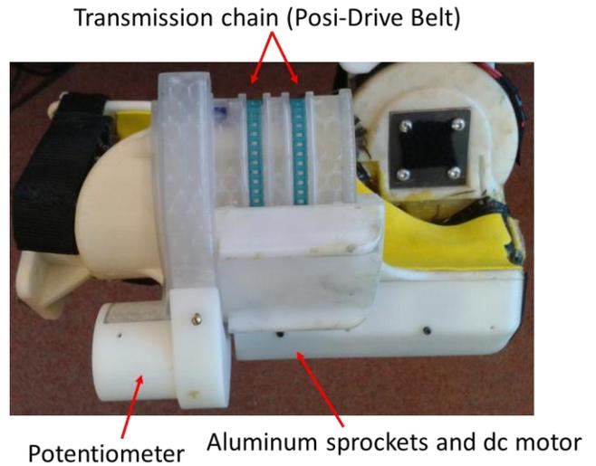
Figure 2 - Pronation/supination mechanism
