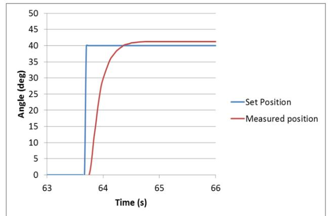
Figure 5 – PID position step response
