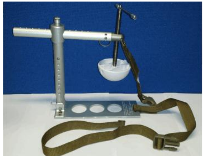
Figure 1: Combat Ready Clamp (CRoC) with hemispherical (3.75 cm [1.5 in] radius) effector head.
