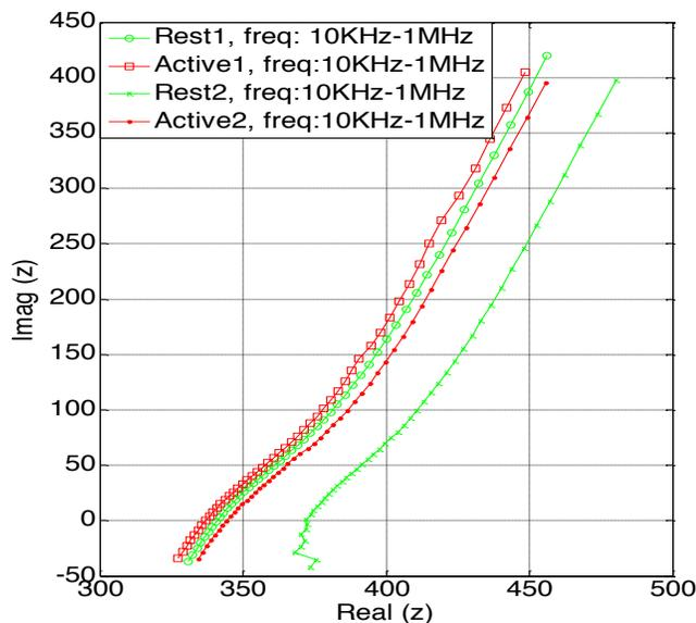
**Fig. 5: Consecutive Rest Active Impedance (10KHz to 1 MHz)**
