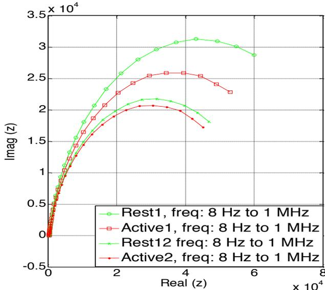
**Fig. 4: Consecutive Rest Active Impedance: 8 Hz to 1 MHz**
