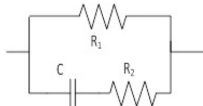
Fig. 1: Three Element RC Model
