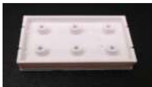
Figure 6. Photograph of printed interconnect mold by MakerBot ready for PDMS molding. The width and length of the chip are 20mm and 30mm, respectively. The inner and outer cylinder diameters are 1mm and 2mm, respectively.
