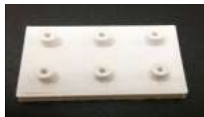
Figure 7. Photograph of printed interconnect by MakerBot. The width and length are 20mm and 30mm, respectively. The inner and outer cylinder diameters are 1mm and 2mm, respectively.
