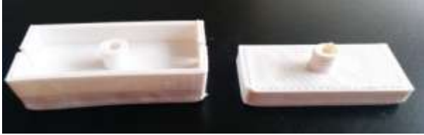
Figure 5. Photographs of printed interconnect (left) and mold (right) by MakerBot. The width and length of the chips are 10mm and 25mm, respectively. The inner and outer cylinder diameters are 1mm and 3mm, respectively.
