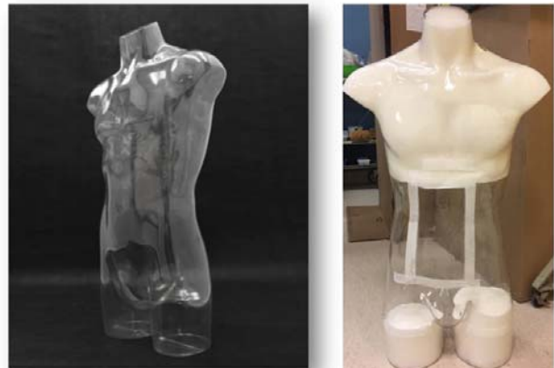
Fig-1: On left (a), empty mannequin; and on right (b), thoracic and femoral portions filled with polyurethane foam.
