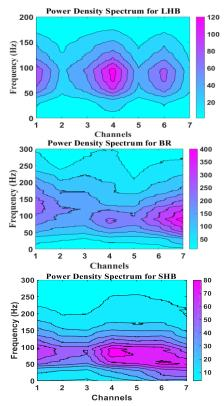
Figure 1: PSD across seven channels for one subject, for three muscles.
