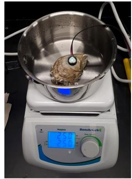
Figure 3: Experimental setup of the oyster heartbeat sensor.
