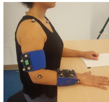
Figure 1: Marker arrangement for the upper extremity, hand, and fingers
