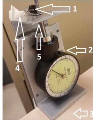
**Fig. 2.** The experimental setup. The spring clamp (1) attached parallel to the operating surface to the force gauge (2) which is clamped to the operating surface (3). The tissue equivalent (4) is pulled downwards by a participant, and this figure shows a support being added to stabilize the spring clamp (5). The force gauge would hold the value prior to the breaking point, which would be recorded as the maximum fastening achieved by a combination of three factors.
