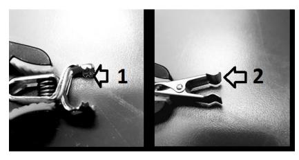
**Fig. 1.** The alligator clip (5) has a toothed jaws, and the spring clamp (2) has two curved surfaces for jaws. Both of these fastening mechanisms are shown in an open position. Pictures were edited in greyscale to show further detail regarding the styles of the jaws.
