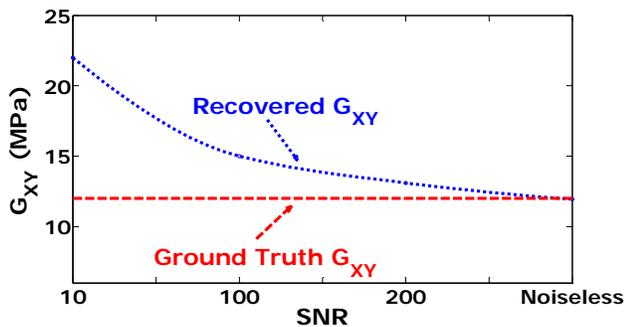
Figure 3: Ground truth and recovered value of in-plane shear modulus by indentation test with different levels of Gaussian noise.
