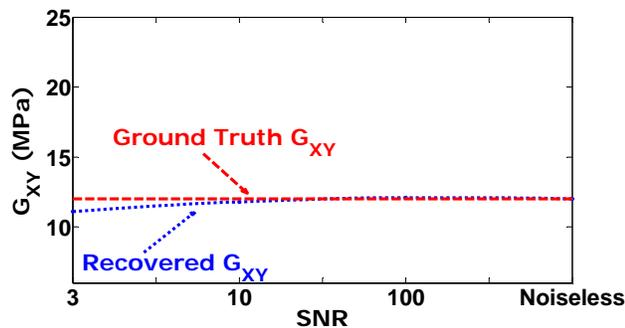
Figure 4: Ground truth and recovered value of in-plane shear modulus by pressurization test with different levels of Gaussian noise.
