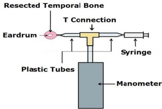
Figure 1: Schematic of pressurization system.
