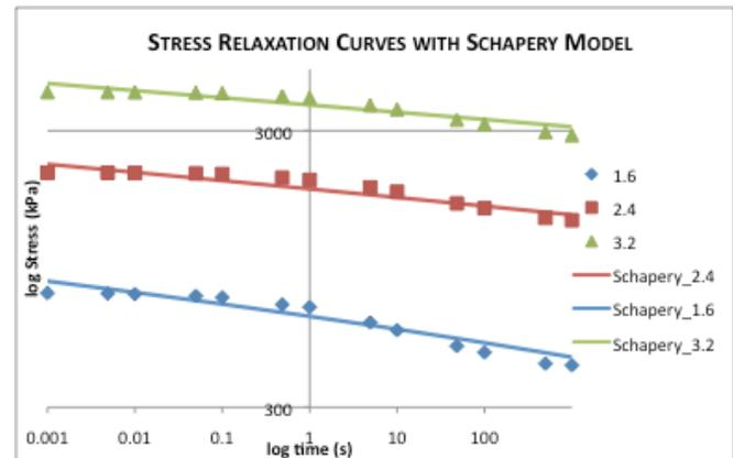
Figure 3: Experimental data with Schapery method model.
