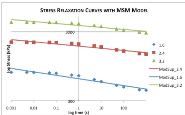
Figure 4: Experimental data with MSM model.
