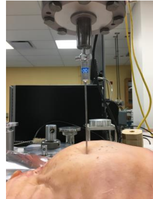
Figure 3. Force puncture test of the Veress needle with the Instron 3366 load frame.
