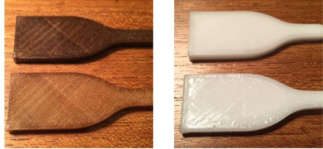
Figure 1: Left, colour difference between unsterilized control (top) and sterilized (bottom) PLA; right, PCL material deformation occurred in the sterilized samples (bottom).
