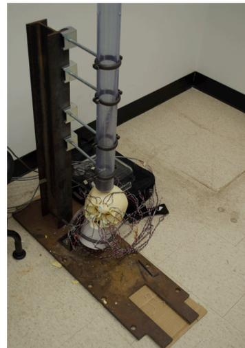
Figure 2: Vertical dropped mass tower apparatus with a specimen in position for an impact at impact site 4.
