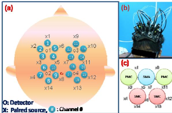
Figure 1. Schematic diagrams the optode locations. (a) The optical fibers were placed on the skull with holders on the custom-made cap (b), Cortical areas covered by the channels as shown in (c).
