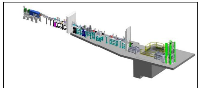
Figure 2: Model of the 05B1-1 Beamline – total length (source to detector) ~29 m [4].
