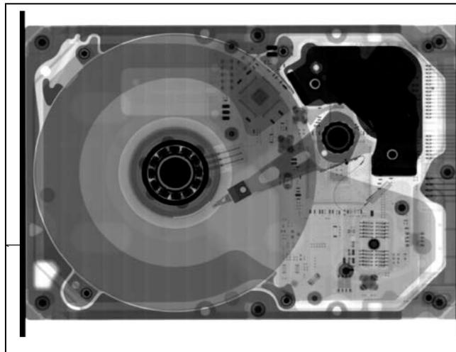
Figure 3: High resolution radiograph of the hard-drive.
