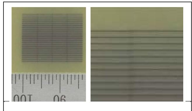
Figure 4: Radio-chromic film (EBT-3) record of the four adjacent micro-beams irradiations (left) (@100 keV) with the beam dose of 250 Gy, scale in mm. Right: zoom-in view.
