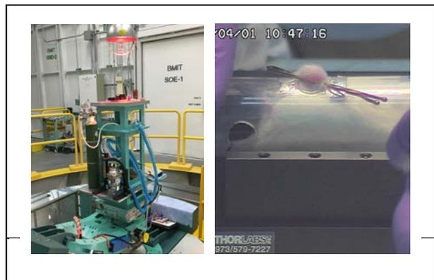
Figure 5: Experimental set-up (left) and close-up of the irradiated tumor (right) for in-vivo treatment of human breast tumor model in mice.
