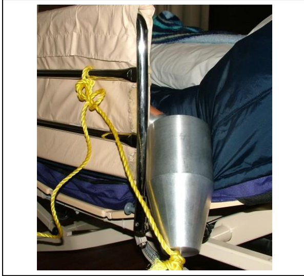
Figure 15.: 12:15 PM. The head drops. Zone 3 test fails.
