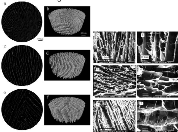
Figure 5: Micro-CT cross-sectional images of scaffolds made with 7% alginate solution and frozen to -80 (a), -50 (c) and -20 (e) degrees. Figure 5(b), (d) and (f) are 3D volume rendering of alginate scaffolds frozen to -80, -50 and -20 degrees respectively.
