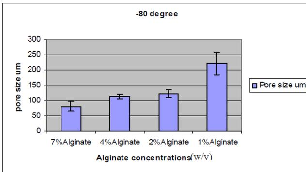
Figure 4: Changes of pore size with different alginate concentrations (1%, 2%, 4%, 7%) at -80 degree.
