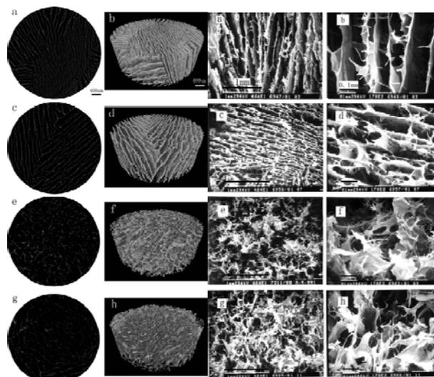
Figure 1: Micro-CT cross-sectional images of 7% (a), 4% (c), 2% (e) and 1% (g) of alginate solutions. Figure 1(b), (d), (f) and (h) show the three-dimensional rendering of the corresponding 7%, 4%, 2% and 1% alginate scaffolds.
