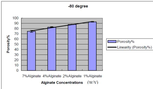
Figure 3: Changes of porosity with different alginate concentrations (1%, 2%, 4%, 7%) at -80 degree. The approximate line shows the linearity of porosity as a function of alginate concentration.
