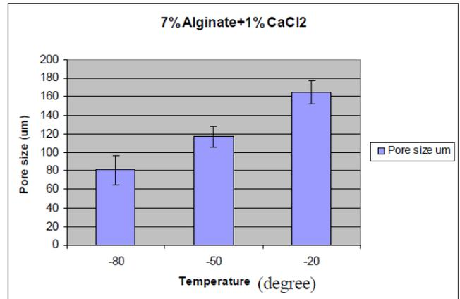
Figure 7: Changes of pore size with different freezing temperature of 7% alginate concentration.
