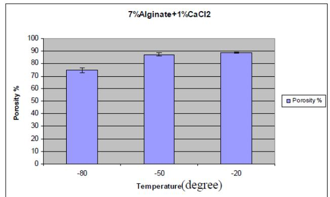
Figure 8: Changes of different porosity of scaffolds made with 7% alginate solution.
