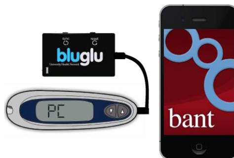
Figure 1: Mobile diabetes self-management system includes Lifescan OneTouch UltraMini glucometer, Apple iPhone or iPod Touch, bluglu hardware adaptor, and bant software application.
