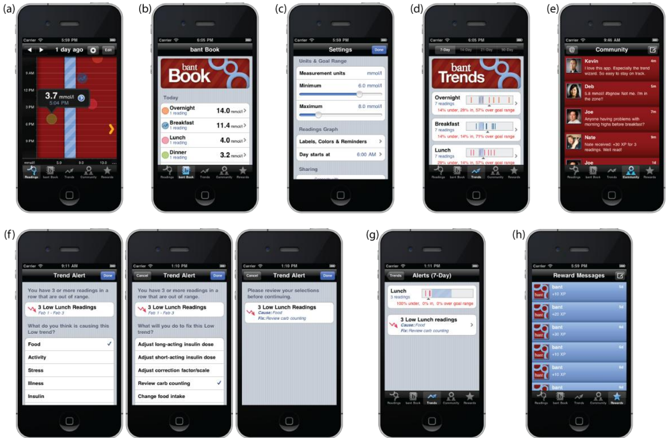
Figure 2: Bant screenshots. (a) Agenda-like BG measurement viewer with goal range. (b) Electronic logbook. (c) Bant settings; ie. adjust goal range, customize measurement contexts, and add reminders. (d) Visualization of 50/30/20 trends. (e) Peer-support via micro-blogging. (f) Alert wizard to assist analysis of consecutive out-of-range measurements. (g) Alert history viewer. (h) Log of experience points earned to be exchanged for gifts.
