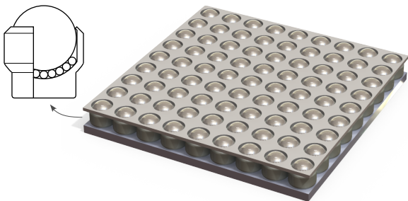
Figure 4: CAD view of an omnidirectional low-friction floor tile, made of ball transfer units
