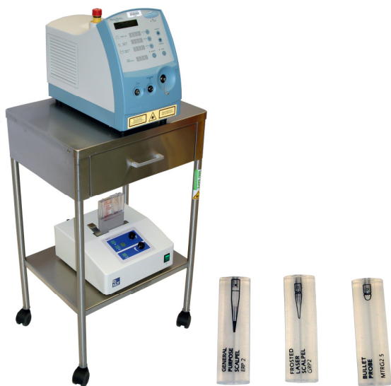
Figure 3: The 980nm diode laser system (left) and sample contact laser tips (right). Not to scale.
