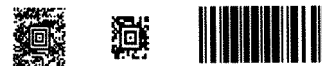
Figure 1: Barcodes: Drug (2D Aztec, ~80 char), Patient ID, (2D Aztec, 7char), Clinician ID (1D Code128, 6 char)
