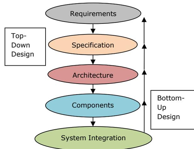
Figure 1.2 Critical levels of abstraction in the Embedded System Design Process [6]
