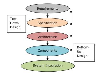
Figure 1.2 Critical levels of abstraction in the Embedded System Design Process [6]
