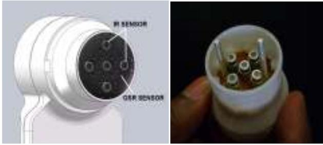
Figure 2: Probe Sensor Head (CAD rendering, Prototype)
