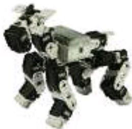
Figure 2 – Robotis Bioloid Dog Configuration
