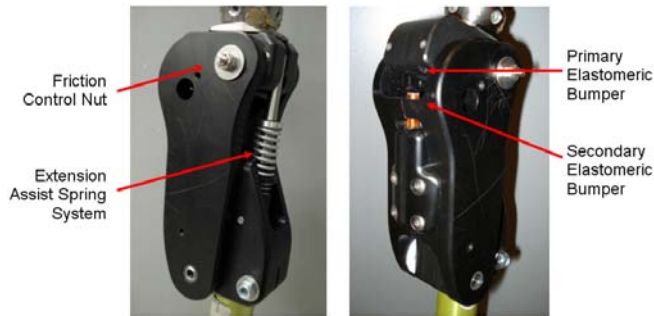
Figure 2: LC Knee Swing-Phase Control Mechanisms
