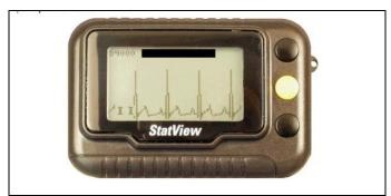
Figure 1: Secondary Alarm notification pager with ECG signal
