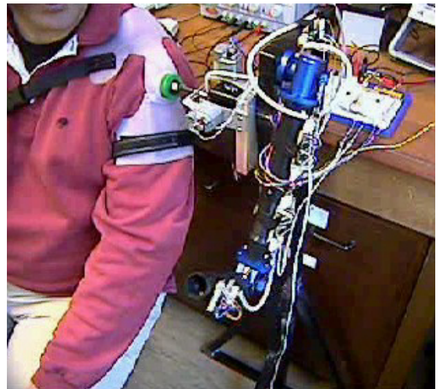
Figure 3 - Arm set up used to explore coordinated joint control. The able bodied volunteer controls the end point of the arm from the motions of his shoulder. The local intelligence of the arm calculates the desired position and each joint moves to them.
