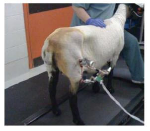
Figure 1: The application of the ISL in measuring sheep joint kinematics during gait
