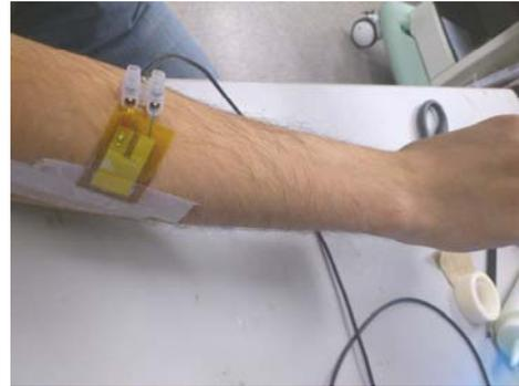
Figure 2: Wearable ultrasonic sensor attached onto a right forearm.
