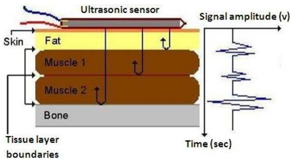
Figure 1: Schematic of the measurement model of tissue thickness.
