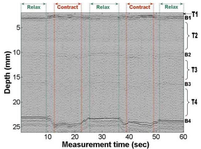
Figure 3: A result of M-mode ultrasound measurement at forearm.
