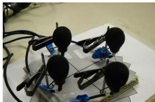
Figure 1: Microphone array set-up
